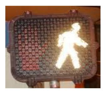
WALK intervals of greater than 7 seconds may be used where the duration of the associated vehicular green interval is long enough to accommodate it. The purpose of the WALK interval is to provide enough time for a group of waiting pedestrians to enter the crosswalk before the flashing DON'T WALK commences.
