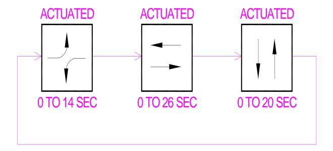
The cycle length will vary from cycle to cycle with a maximum cycle length for this example of 60 seconds. Fully-actuated controllers offer the most sophisticated timing features and capabilities so the remaining discussion centers on these types of controllers.
