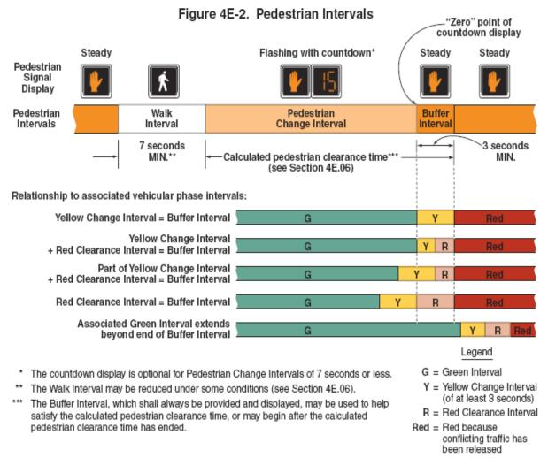
Countdown pedestrian signals, which are now required by the MUTCD when the pedestrian change interval is longer than 7 seconds, display the number of seconds remaining until the termination of the pedestrian change interval.
