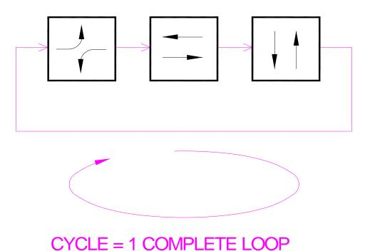
If the three phase combinations in the above diagram each last for 30 seconds, then the cycle length for this signal is 90 seconds. A cycle is sometimes referred to as a "dial" since, in old electro-mechanical controllers, a rotating dial was used to control the timing of the various signal displays. The amount of time during which a particular phase has a green indication (either ball or arrow) is known as the "green interval" for that phase
